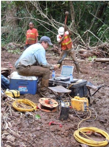
Each seismic array consisted of 48 geophones with an inter-geophone spacing of 3 meters, for a total array length of 141 meters. The travel times of the P-wave energy were manually picked for each shot using Pickwin (OYO Corporation). The travel-time picks were imported into Plotrefa (OYO Corporation) for modeling.
