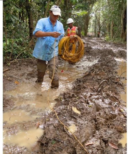
MASW data were recorded using a Geometrics Smartseis ST seismograph and 4½-Hz geophones. Each seismic array consisted of 24 geophones with an inter-geophone spacing of 1.5m, for a total array length of 34.5m. Data were processed using SurfSeis v. 2.0. Seismic Refraction data were recorded using two Geometrics Geode and 40-Hz geophones.
