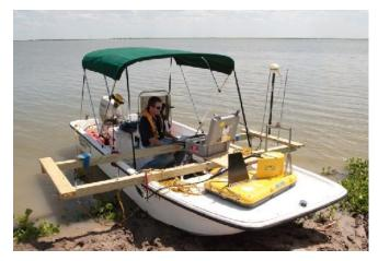
Bathymetric and sub-bottom surveys were conducted within a clay settling pond at a Phosphate mine in Central Florida. Prior to the geophysical survey, a depression or slump had formed along the northern dam of the pond. The purpose of the study was to map various sediment layers within the pond to help determine if the depressions or slumps were related to sinkhole activity or if they were related to dredging activity.
