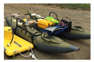
GeoView, Inc. conducted a bathymetric study within the western portion of pond at a limestone mine in Marion County, Florida. As part of a roadway expansion project, the western portion of the pond was to be infilled. The purpose of the study was to map the water depth in order calculate slope analysis and fill volume.
