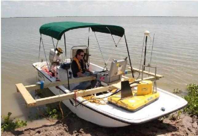
Bathymetric and sub-bottom surveys were conducted within a clay settling pond at a Phosphate mine in Central Florida. Prior to the geophysical survey, a depression or slump had formed along the northern dam of the pond. The purpose of the study was to map various sediment layers within the pond to help determine if the depressions or slumps were related to sinkhole activity or if they were related to dredging activity.
