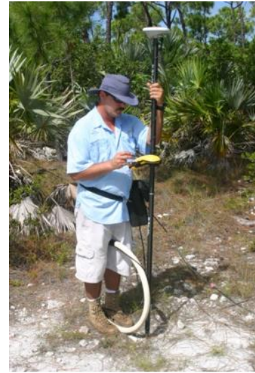
EM 34 Being Used to Collect Conductivity Measurements with GPS Positioning
