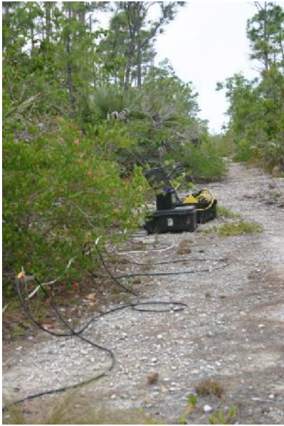
Field Deployment of ERI Equipment
